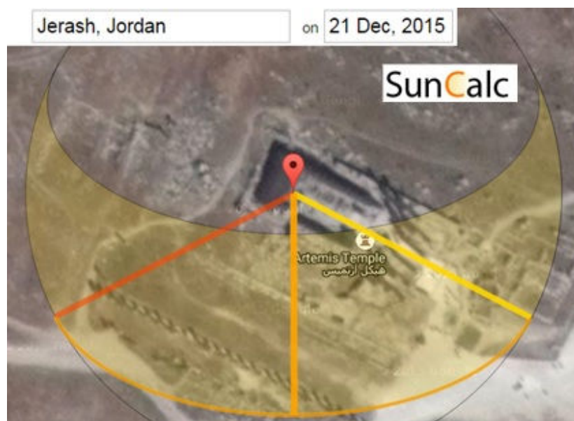
Figure 7: Sunrise and sunset directions on the winter solstice as given by SunCalc.net.
